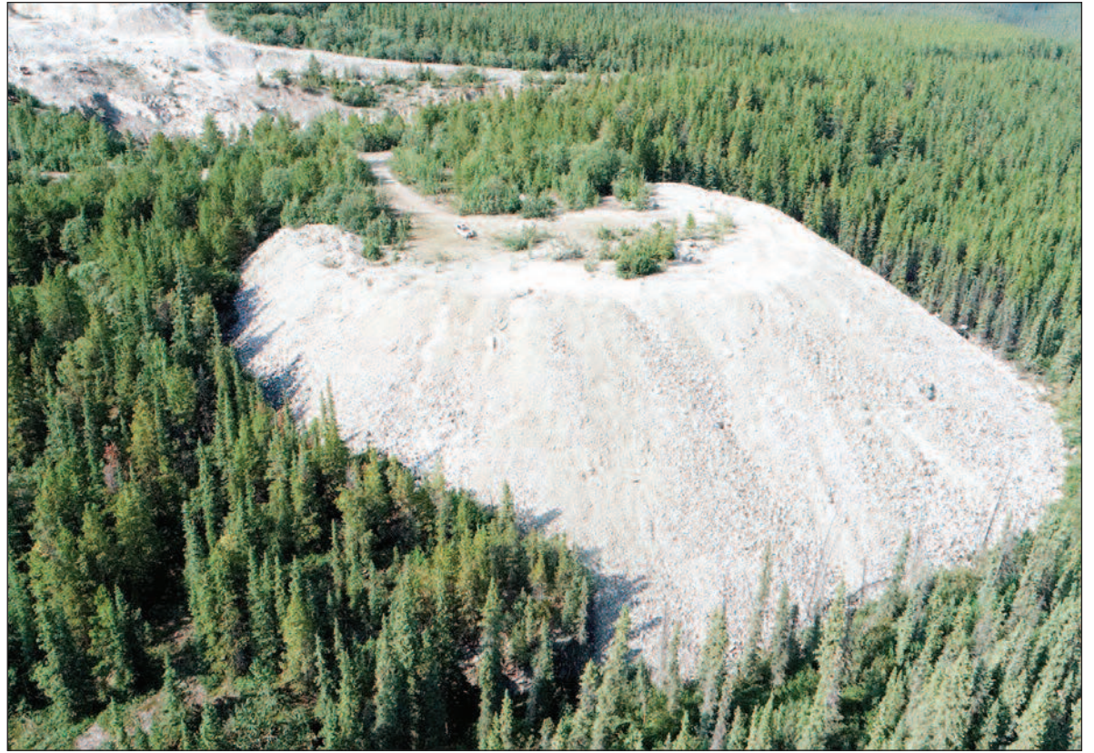
Waste rock pile at Arctic Chief. The car on top provides a rough idea of the large volume of rock that never went to the mill, discarded because it contained insufficient copper.
